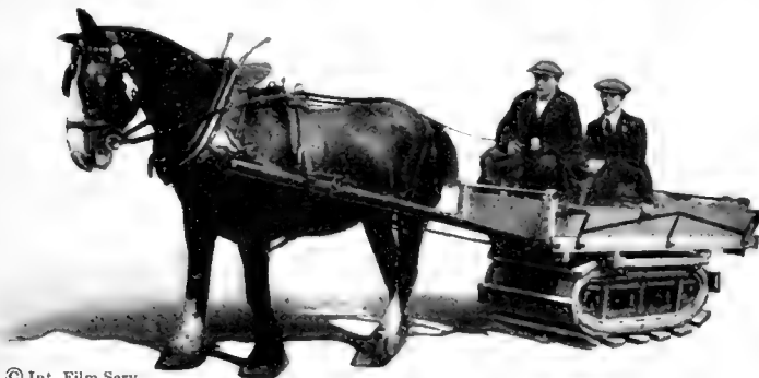
© Int. Film Serv. A caterpillar tread attached to an English delivery cart enables it to go anywhere regardless of the condition of the roads
